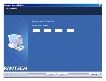
8 Enter the **Serial Number** for the EntraPass Special Server or Software. The information is located in the CD pocket. Make sure to enter the correct digits. The **Next** button is only enabled if the installation code is correct.
