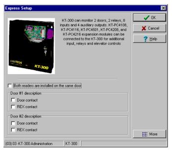
2 Specify if **Both readers are on the same door** if this is applicable. If two readers are installed on the same door, the REX contact option is disabled.
